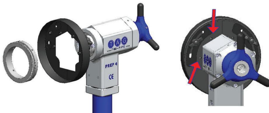
Figure 4-1 Installing the protector and ring gear
