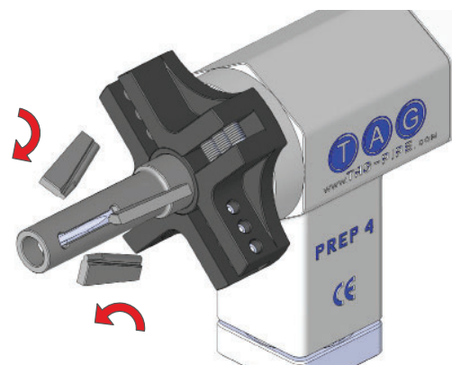
Figure 3-7 Installing the locking jaws
