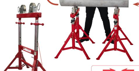
Various height holes enable the operator to fix the stand at the required working height using the safety locking pins
