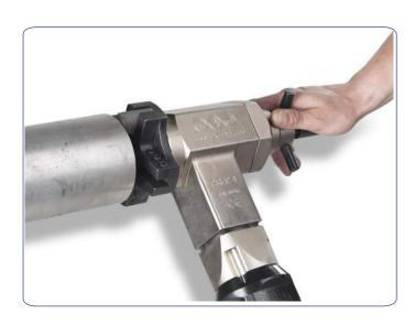
The Jaw system itself consists of 3 equilaterally positioned machined jaw segments, retained and locked on an inner, 'grooved' expansion shaft. These grooves keep the jaws held securely in position, unlike other systems that use a metal or rubber bands for jaw retention.
