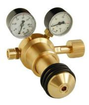
The pressure regulator is available in version for working pressure up to 100 bar or up to 200 bar. The working pressure is infinitely adjustable with the handwheel between 10 - 100 bar, resp. between 10 - 200 bar. For an easy pressure adjustment the handwheel shows at the front a hexagon, so that the pressure adjustment can also be made by means of a socket wrench 8 mm.
